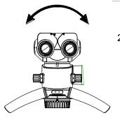
2 Friction adjustment knob for tilting motion (left/right) of the main lens of the microscope
