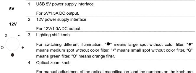
For manual adjustment of the optical magnification, and the numbers on the knob are magnification factors.
